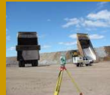
Measuring trucks to estimate their coal carrying capacity
